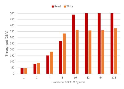
Figure 4. FIO throughput scaling with a very large number of DGX A100 systems
