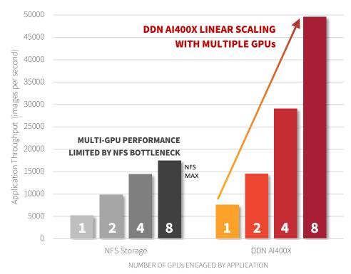
Figure 7. Scaling PyTorch application performance on DGX system
