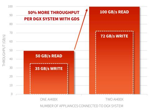
Figure 3. Scaling throughput performance on DGX system with AI400X appliances
